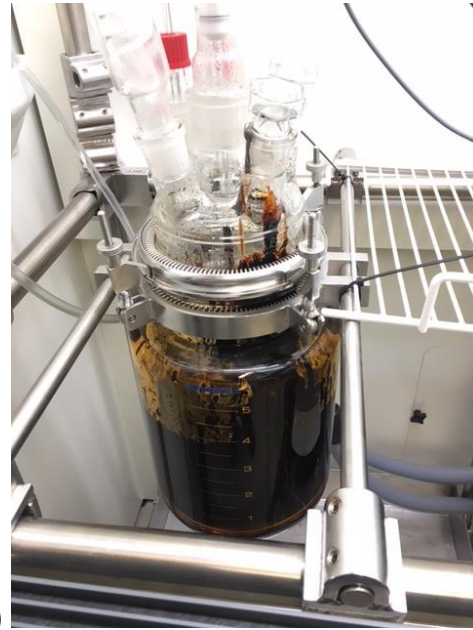
(a) Lab-scale equipment (reaction V=100 ml) & (b) Scale-up reactor for synthesis performance of magnetic nanomaterial (reaction V=4L)
