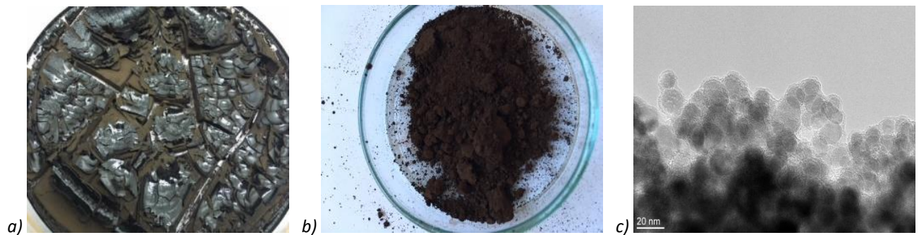
Figures 2: (a) Scale-up prepared, stabilized and functionalized \gamma\text{-Fe}_2\text{O}_3 magnetic nanoparticles (SUP F-MNP T: A_sAM): (a) dried, (b) crushed and finely powdered; (c) TEM image of nanoparticles
