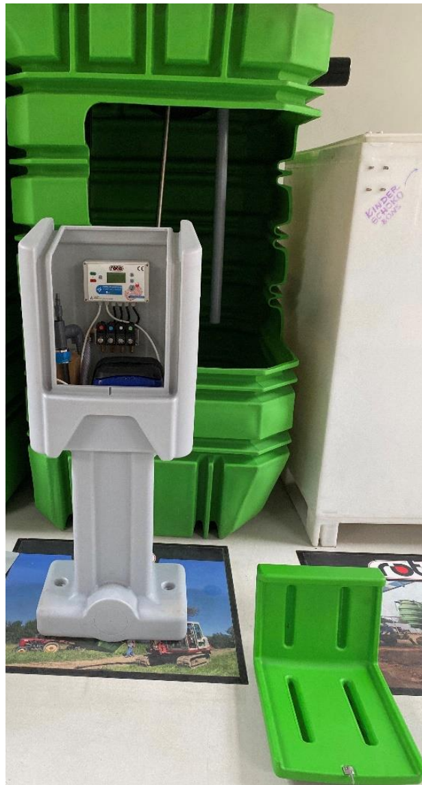
Figure 2: Cylindrical cartridge in preliminary cartridge housing, produced from (LMDPE) / HD UV polypropylene-copolymer
