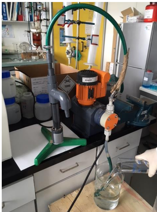
Figure: Testing setup with preliminary cylindrical cartridge filled with magnetic nanomaterial (MNs)
