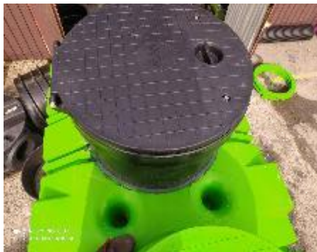
Figures 3: PROTOTYPE MBR REACTOR – Adjusted: (a) chambers, (b) inlet and outlet openings, (c) reactor wall, (d) opening for membranes, (e) lids, & (f) sampling vessel
